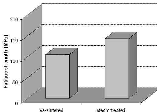
**Figure 2. Comparison of fatigue strength**
