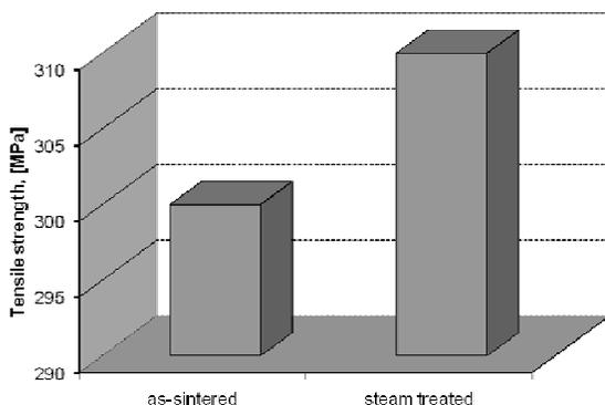
**Figure 1. Comparison of tensile strength**
