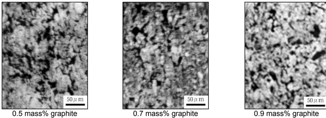
**Figure 5. Microstructures of steam treated specimens**
