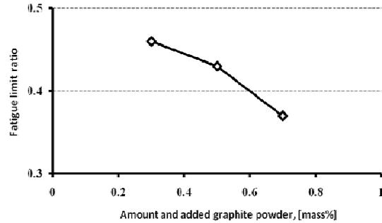
**Figure 7. Relationship between amount of added graphite and fatigue limit ratio of steam treated specimen**
