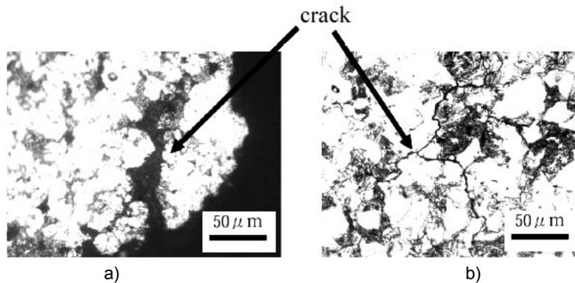
**Figure 8. Appearance of crack propagation in static (tensile) destruction (a), and fatigue failure (b)**
