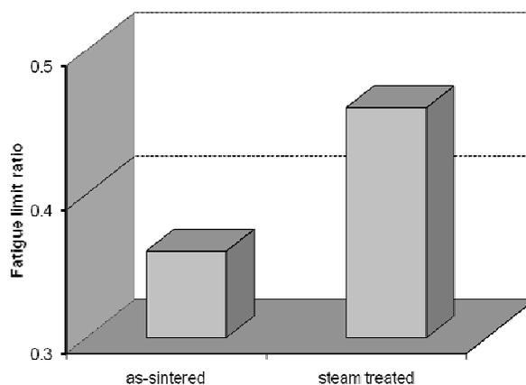
**Figure 3. Comparison of fatigue limit ratio**
